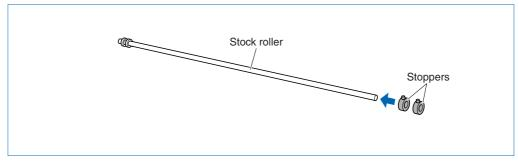
Position the stock roller with the stoppers towards the front, and place the other stock roller toward the rear to suit the roll-medium size.
