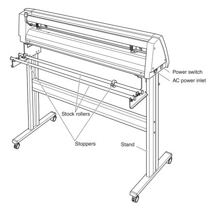
AC power inlet Power switch Stand Stock rollers Stoppers
