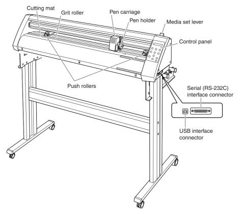
Cutting mat; Cutting or plotting is performed on this mat.Grit roller; Feeds the medium backward or forwardPush rollers; Pushes the medium against the grit rollersPen carriage; Moves the cutter pen to the left and rightPen holder; Holds the cutter pen and moves it up and down
