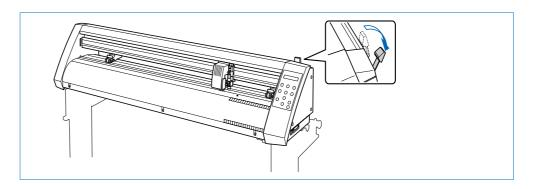
Place the roll medium on the stand stock rollers, and then pass the leading edge of the medium from the back of the cutting plotter so it emerges from the front, while making sure to remove any slack in the medium conveyance path.
